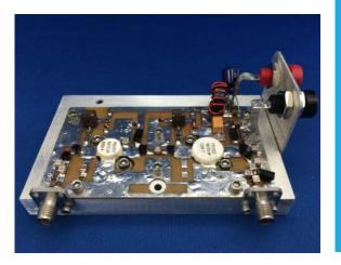
(T) TB224 featuring the SP201: 30-512MHz, 1.0W P1dB, 10dB, 12%, 28VDC
