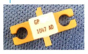
**GP1001:** 10W, 2.5GHz, 11dB, 50%, 28VDC **GP2001:** 20W, 2.0GHz, 11dB, 65%, 28VDC **GP1441:** 10W, 2.5GHz, 11dB, 35%, 48VDC **GP2441:** 40W, 2.5GHz, 11dB, 55%, 48VDC
